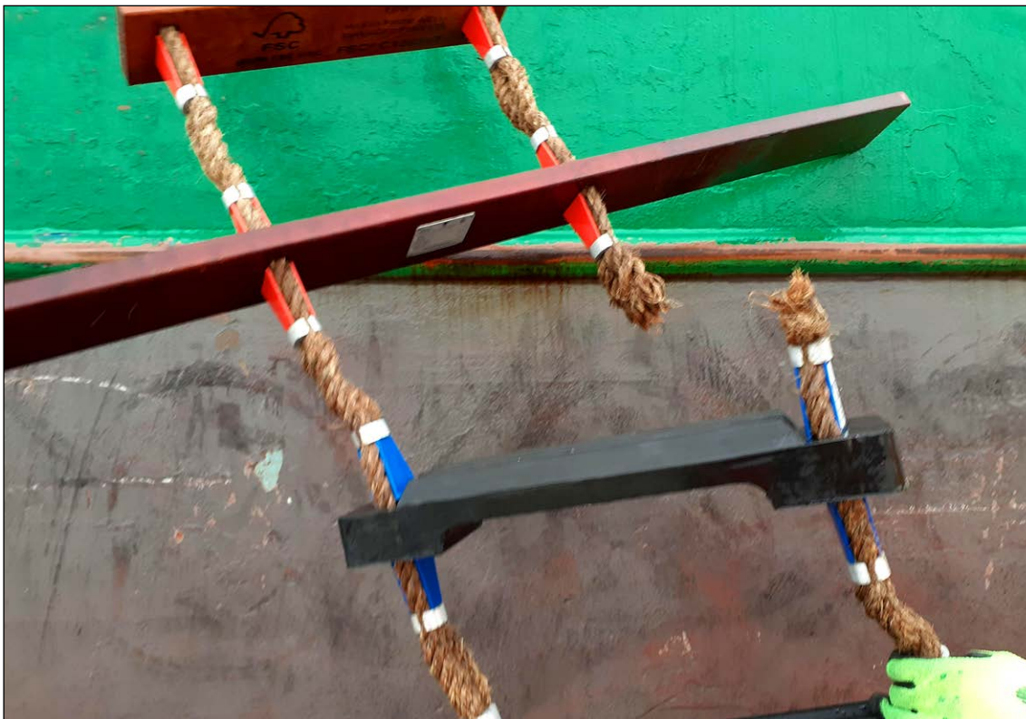
Figure 2: Example of a failed pilot ladder
