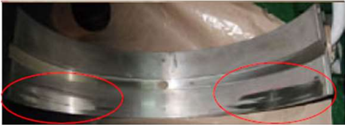
Upper main bearing shell with signs of spark erosion
